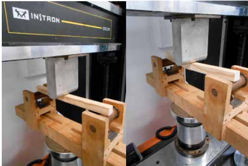
Figure 1. 3-point bend testing of Radiata pine samples, before and after failure.
