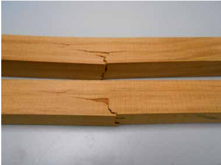
Figure 4. Failure of samples of Lignia batch BG, showing crack deflection.
